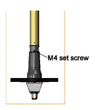
Secure the assembly using the M4 set screw provided with the antenna (2mm Allen Wrench)
