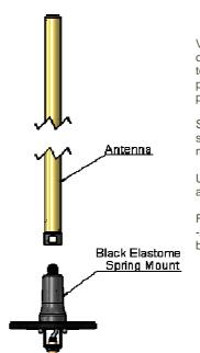
Visually inspect the inner part of the connector of the antenna to make sure no sand, dirt or plastic material will prevent proper electrical mating.
